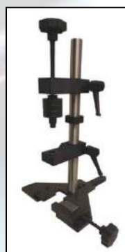
Measuring vice, comparator base, vice to unscrew the injector nozzle, press for CR12.1
