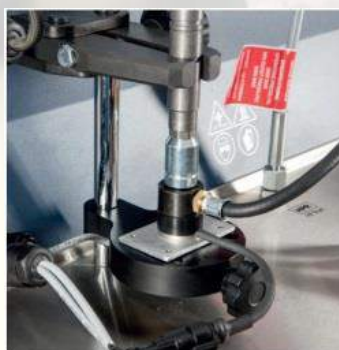
RPSSENSOR – injector response time sensor
