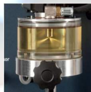
iPSC – pressurised spray observation chamber
